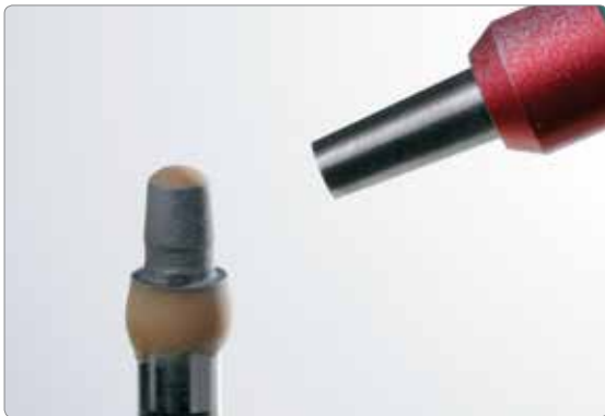
The instructions of the implant manufacturer must be observed. Carefully blast the bonding surface with max. 50 µm and 1-2 bar (15-29 psi) pressure.
