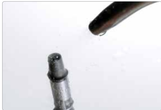
Remove silicone and subsequently clean in an ultrasonic bath or with the steam jet.
