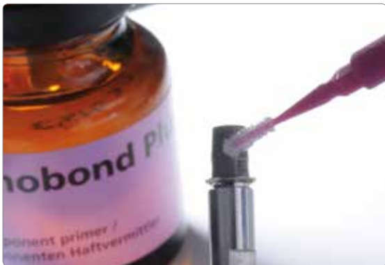
Apply Monobond Plus on the cleaned bonding surface and allow to react for 60 s. After the reaction time, dry the remaining residue with water- and oil-free air.
