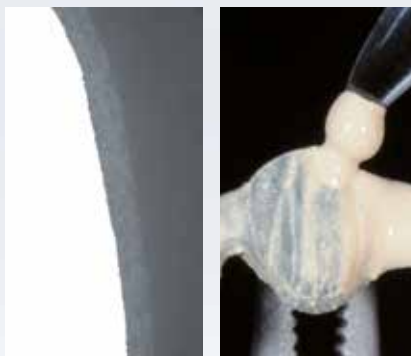
Highly homogeneous opaquer layer (SEM photo). Optimal material combination for opacity and masking strength
